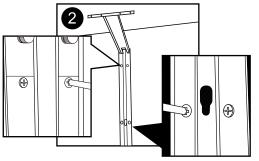
2. Replace the previous hanging bracket with the Vertical Frame, using the same holes and the new Tapping Screws to fix the Vertical Frame to the wall. Suggest that the top of the Vertical Frame should also be fixed to the wall for safety and better performance.
